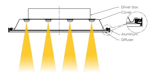
LEDs aim directly at the diffuser
